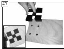
Place floating brackets onto blades aligning holes in blade with the floating bracket. Make sure that the floating bracket does not hang over the edge of blade (see insert).
